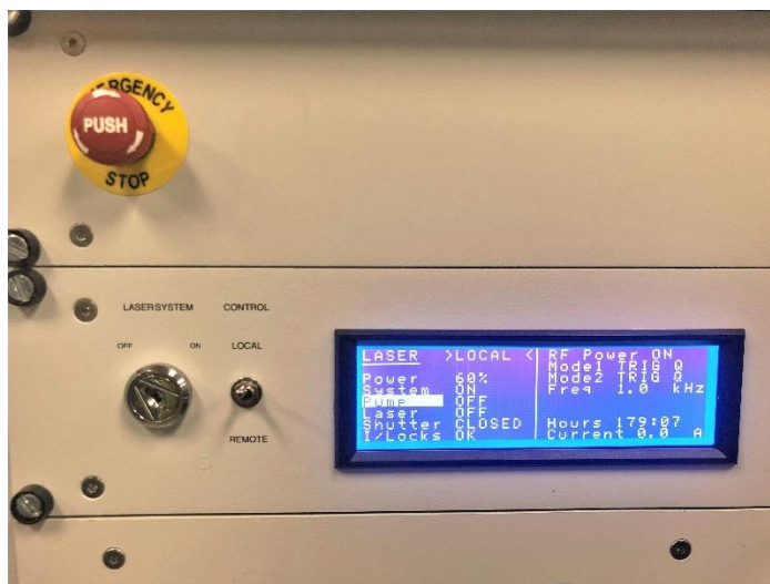
Figure 3 Power Supply Control Panel
