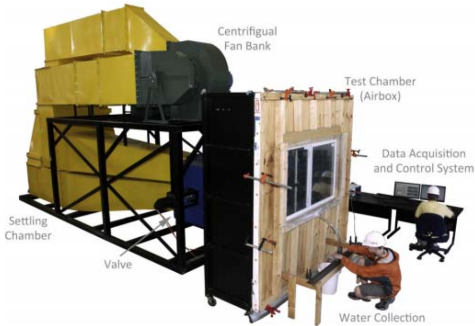
Figure 1 - Layout and components of the High Airflow Pressure Loading Actuator
